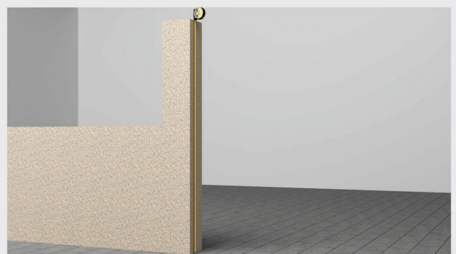
5 Mesurer en haut. Retenir la plus petite mesure; Consider the smallest distance between pillars (bottom, middle, top);
